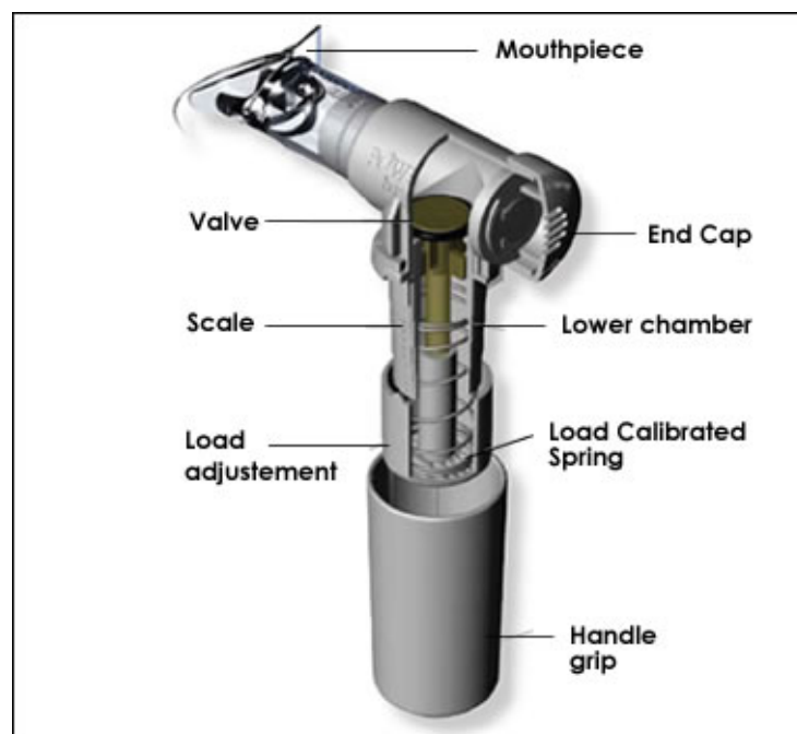
Exploded view of POWERbreathe Medic
